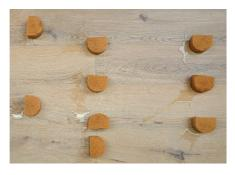
**Test 2**: a sponge test with wet sponges on the joints of an installed floor for 24h.
