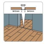
Install the laminate **according to the installation instructions**, with an expansion gap of 8-10mm. Do not install laminate under (fixed) heavy objects such as a bathtub, integrated cabinets,... Install heavy or fixed furniture <u>before</u> you install the floor.
