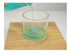
**Test 1**: a test with a cylinder filled with water (Nalfa surface water test) that is put on the joints of an installed floor for 24h to check water intrusion.
