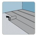
➤ **Underlay**: The installation starts with a BerryAlloc underlay with integrated moisture barrier. Use the **Excellence Impact Plus** underlay or **Excellence Plus** underlay for the best result (read the *BerryAlloc Underlay Guide for more details*). Even if the laminate is water-resistant, a moisture barrier is necessary!
